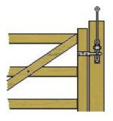
An alternative ' hook and eye' style gate fasteners are also easily opened and closed from horseback.
